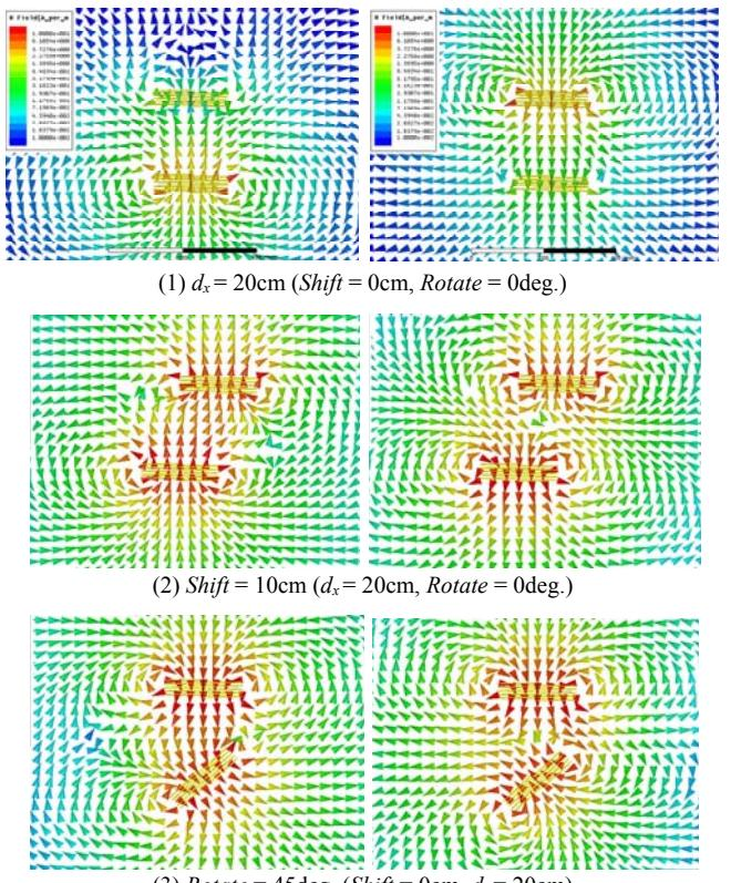
Fig.15 Magnetic field analysis near two resonant coils.
