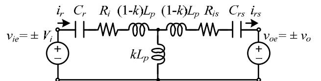
Fig. 5 Equivalent circuit with coupling coefficient  $k$ .
