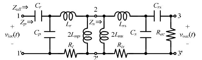
Fig. 10 Multi-resonant circuit.
