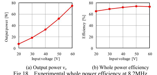
Fig.18 Experimental whole power efficiency at 8.2MHz.
