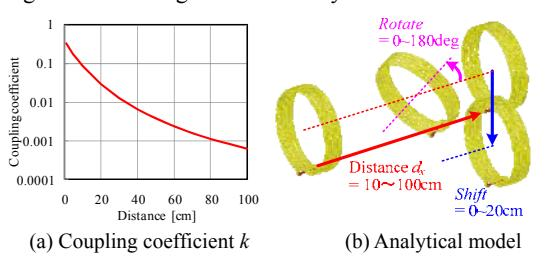
Fig. 7 Coupling coefficient  $k$  for two resonant coils.
