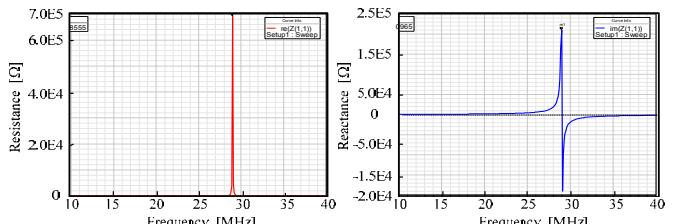
Fig. 8 Impedance characteristics of a resonant coil.
