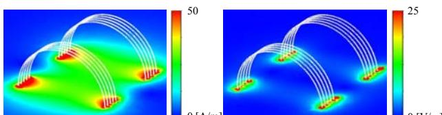
Fig. 6 Electromagnetic field analysis near two resonant coils.
