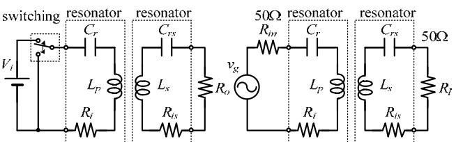
(a) Switching WPT system      (b) Low efficiency WPT system
