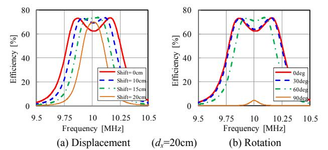
Fig.17 Whole power efficiency characteristics by SCAT.
