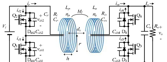
Fig. 3 Multi-resonant ZVS wireless power transfer system using electromagnetic field resonant coupling coils.
