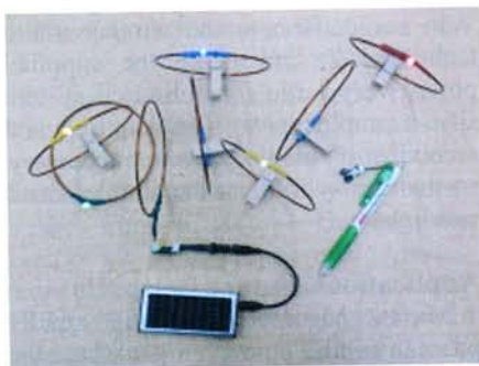
Fig. 7: Scene of proving experiments of the wireless power transfer system using the DC-resonance method
