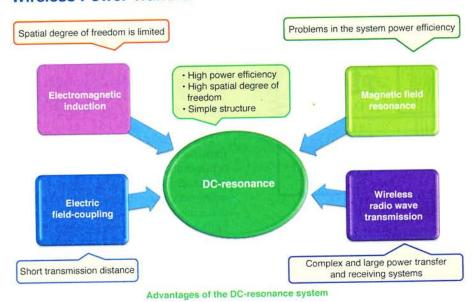
Fig. 6: Merit of DC-resonance system
